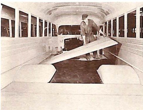
Plywood over steel floor. This optional extra provides still further insulation against cold and road noises.
