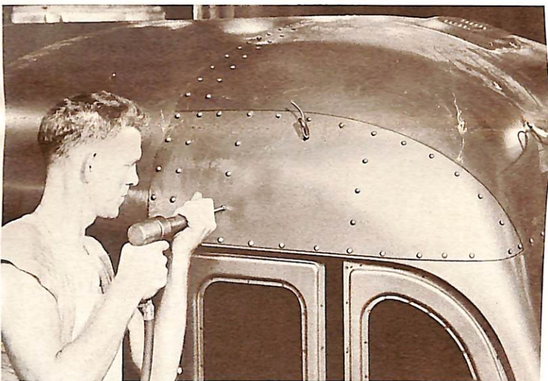
Closely spaced riveting is another example of Superior's emphasis on safety and durability. This view shows riveting of an additional corner panel, for 3-panel thickness over the entrance.
