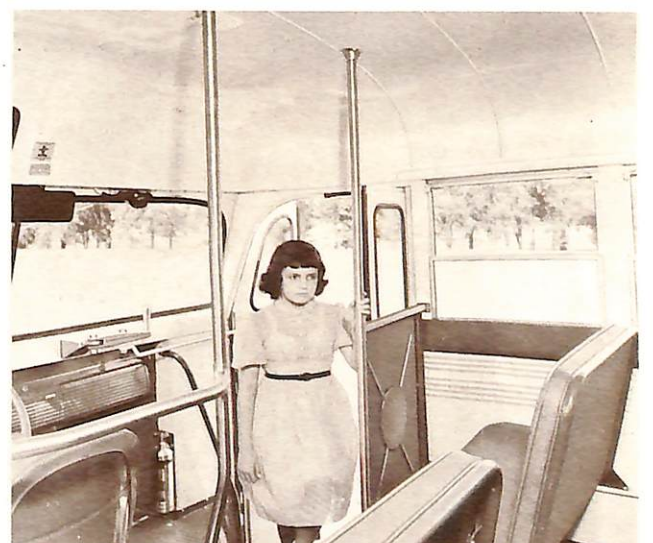
Sturdy stainless steel stanchions increase safety of children entering or leaving bus. Tubular rail behind driver's seat safeguards driver from accidental interference. Rigid decency panel, from entrance stanchion to wall, shields entrance way.
