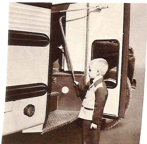
Easy-to-reach hand rail helps even the smaller children get on or off safely. Non-slip steps. Automatic step-well light.
