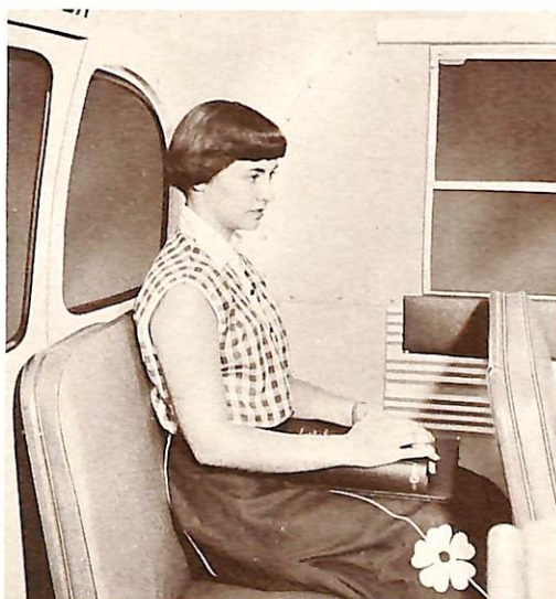
Extra headroom at rear eliminates "bent-neck" posture, cuts down possibility of head injury from rear crash. Distance from back seat cushion to roof panel exceeds state and national requirements.
