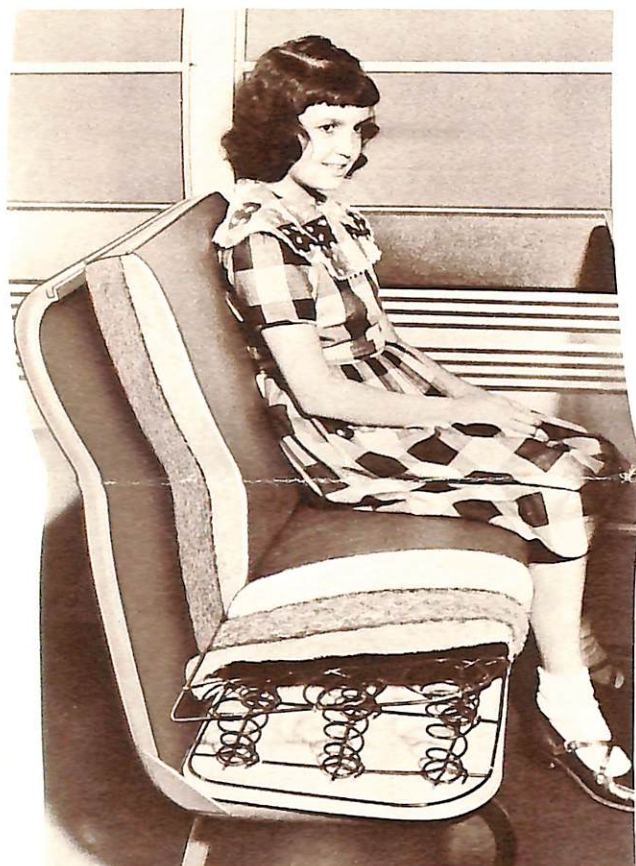
Restful, wear-resistant seat construction: Thick, double-padded cushions and backs. Heavy-duty, plastic-coated upholstery is easy to clean, withstands temperature changes, resists scuffing, scratching and stains. Cushion has plywood base, heavy-duty springs. Sturdy tubular steel frame.
