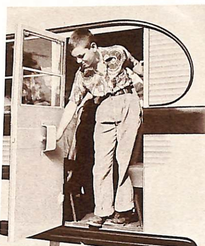
Side emergency door blends with exterior styling. Same type hinge, double catch, release guard, and rubber seal as rear door. Available when specified.
